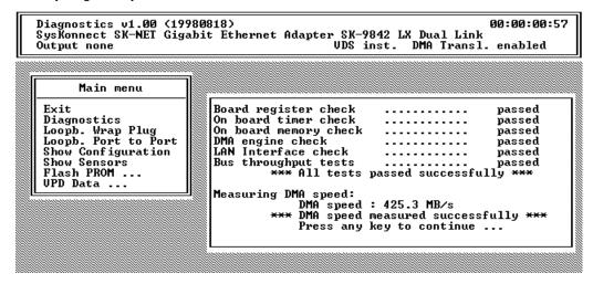
Fig. 7. Typical screen display following a successful test
